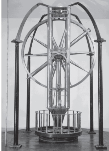
Fig. 2. The Palermo Circle. This meridian circle was constructed by Jesse Ramsden (1730–1800), the greatest of the eighteenth-century instrument makers. It was completed in 1789 after almost two years of intense work. The telescope has a 7.5-cm objective lens; the altitude scale (5 feet in diameter) was read with the aid of two diametrically-opposed micrometer microscopes while the azimuth scale (3 feet in diameter) was read by means of a micrometer microscope.
